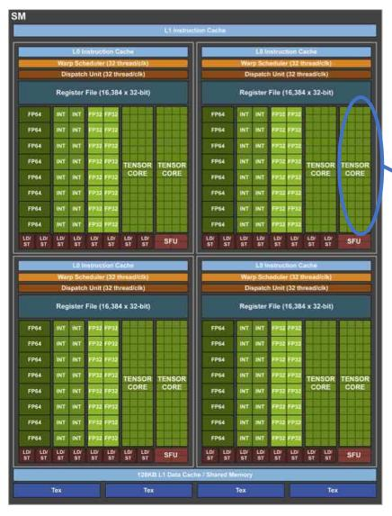
15.7 TFLOPS Single Precision7.8 TFLOPS Double Precision125 TFLOPS for Deep Learning (Tensor cores)
